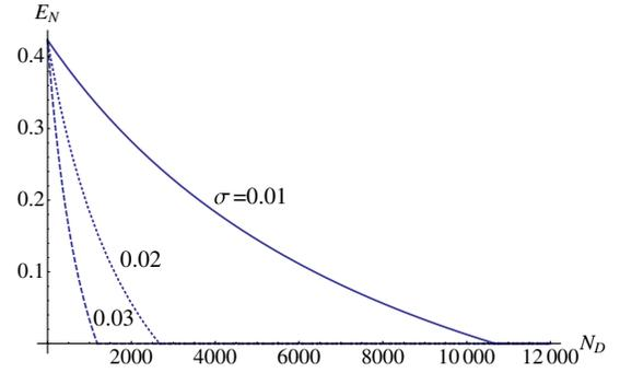
FIG. 3 (color online). Entanglement in the final state as a function of the displaced photon (or phonon) number  $N_D = |\alpha|^2$ , for different values of the phase noise standard deviation  $\sigma$ . Phase noise limits the size of the displacement for which entanglement can be shown. Here  $y = 0.1$ ,  $N_{\text{in}} = 1$ , and the other parameters are the same as in Fig. 2.
