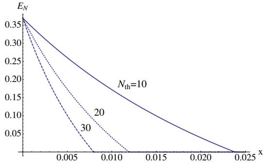
FIG. 4 (color online). Entanglement in the final state as a function of the mechanical noise parameter  $x = \gamma/G$ , for different values of the bath mean phonon number  $N_{\text{th}}$ . The values of the other parameters are  $N_D = |\alpha|^2 = 5000$ ,  $r = 0.5$ ,  $y = 0.1$ ,  $N_{\text{in}} = 1$ ,  $\sigma = 0.01$ , and  $\eta_1 = \eta_2 = \eta_c = 0.8$ .
