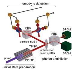
FIG. 1 (color online). Experimental setup. Type II parametric down-conversion in a PPKTP crystal generates the two-mode squeezed vacuum state in two polarization modes. Each mode is subjected to the annihilation operator realized by an unbalanced beam splitter and a single photon detector. The prepared distilled two-mode squeezed state has higher squeezing and entanglement, as verified by homodyne detection. SPCM, single-photon counting module; PBS: polarizing beam splitter.
